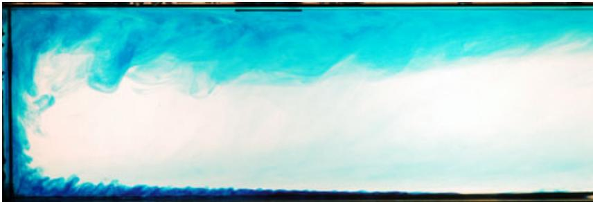
Figure 3.27: Horizontal convection experiment where the left side of a tank is heated at the bottom, and the right hand side (not shown) is cooled. Water rises, primarily along the left hand wall. <http://rses.anu.edu.au/gfd/AR2005/index.php?p=ar05res>
